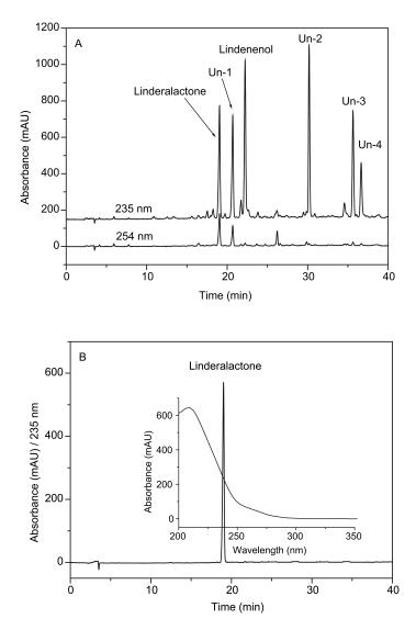
**Figure 2.** HPLC chromatogram of crude extract from *Radix linderae* and HSCCC peak fractions. Column: SPHERIGEL ODS  $C_{18}$  column (250 mm × 4.6 mm I.D., 5 µm); mobile phase: acetonitrile and water in gradient mode (acetonitrile : water (v/v) from 30:70 to 84:16, in 30 min); flow rate: 1.0 mL min<sup>-1</sup>; detection wavelength: 235 nm and 254 nm; (A) crude extract from *Radix linderae*; (B) peak I; (C) peak II of Fig. 3.
